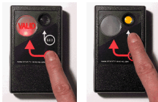
Left: The Authenticator's LPI reader. Right: The Authenticator's micro-text / micro-image illuminated viewing lens.
