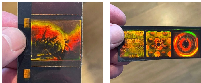
Left: Bayfol HX photopolymer 3Digital reflection dot-matrix hologram of an electron microscope image of a vegetable mite. Right: Bayfol HX photopolymer dot-matrix digital reflection security holograms.
