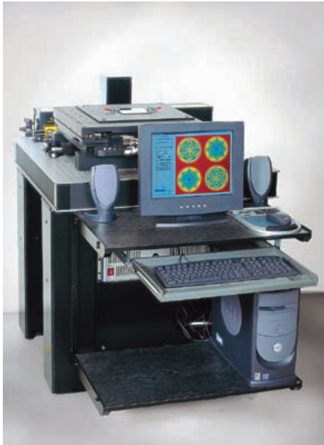
The Lightgate 1270, 1997, utilising a 442nm helium cadmium laser.
