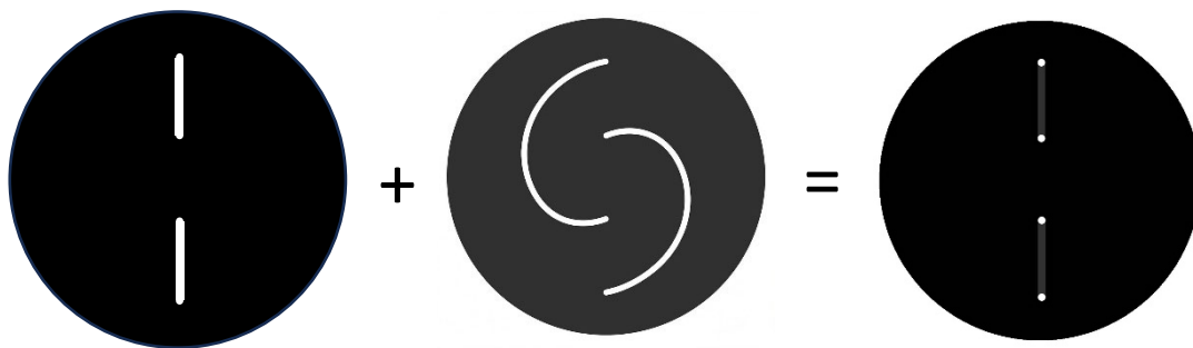
The mask positions relative to each other for the selection of four beams.
