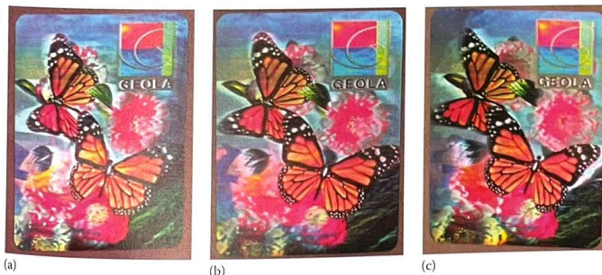
FIGURE 21.22 Embossed 28 × 38 mm hologram produced by OAO NPO "Krypten" from DWDH original made by Geola Digital, ua—views from left, center and right (a–c). (Photograph by Laura Zacharovaite.)
