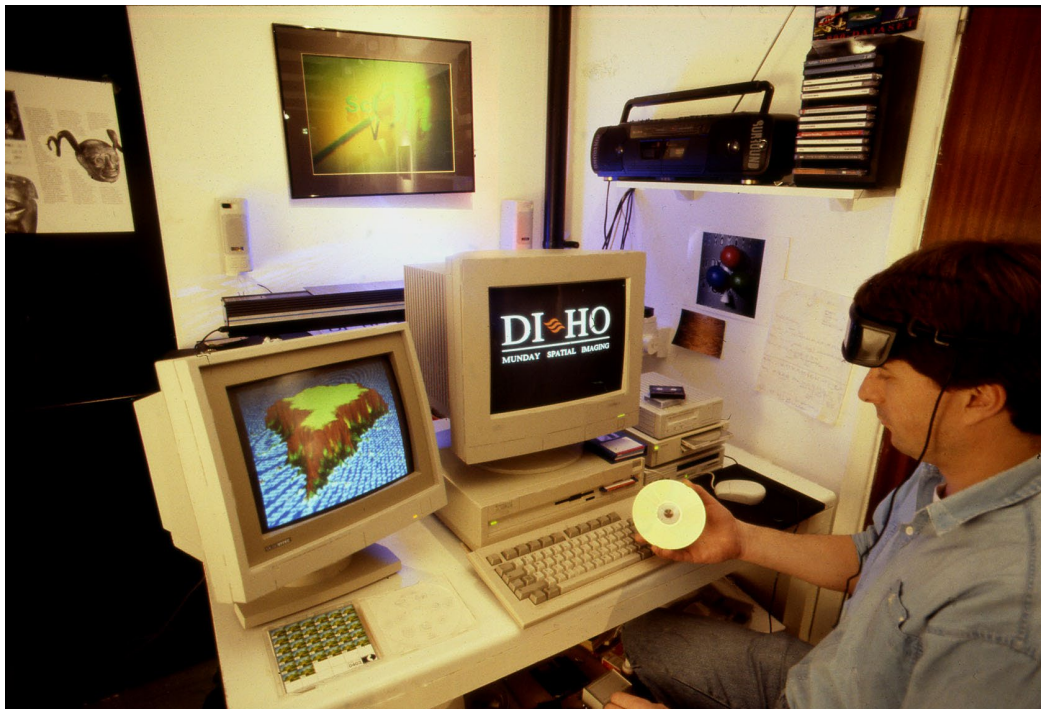
Rob Munday controlling his DI-HO (Digital Input – Holographic Output) holographic stereogram mastering system. He is pictured in front of his Commodore Amiga 3000 system holding a Kodak Photo CD. To the right are CD ROM drives and SyQuest removable hard-disk cartridge drives. On the monitor to the left can be seen my image Mandelbrot Mountain, a digitally produced full colour 3D stereogram of a mountain scene in the shape of a Mandelbrot fractal which was computer generated using the unique fractal landscape generating program VistaPro by Virtual Reality Laboratories.
